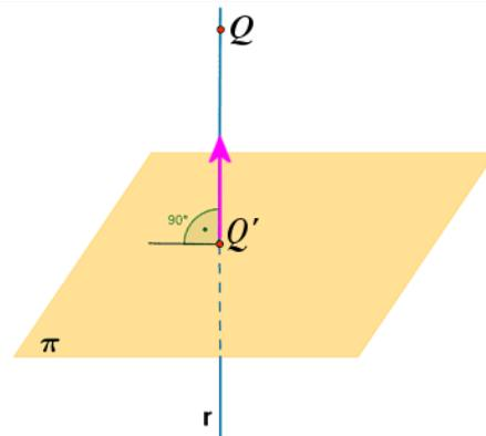
$$\left. \begin{array}{l} \vec{v}_r = \vec{n} = (1, 2, -3) \\ Q(-1, 0, 1) \end{array} \right\} \Rightarrow r \equiv \left. \begin{array}{l} x = -1 + t \\ y = 2t \\ z = 1 - 3t \end{array} \right\}$$
